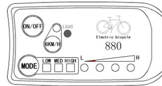
Hold **MODE** button long to startup the lights (the controller should have the function of headlight driving output or built-in meter headlight driving output function), **LIGHT** indicator lights. Hold **MODE** button again to turn off vehicle headlights, and the **LIGHT** indicator is turned off.
