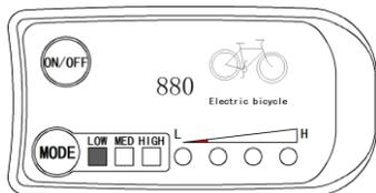
Hold **MODE** button shortly to switch 1-3 file gear, LOW is for the minimum power gear, MED is for the middle power gear, and HIGH is for the highest power gear. Each startup will automatically restore the gear shutdown last time.
