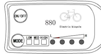
When battery power capacity is greater than 80%, all 4 LED indicator are lit. When the battery capacities drop, the indicators are off in order. When the power capacity is less than 20%, the last indicator is flashing (L side). When the controller is under-voltage protection, all 4 LED indicators are power off, which means that the vehicle is currently shutdown due to low voltage.
