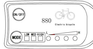
Hold **MODE** button long to startup the lights (the controller should have the function of headlight driving output or built-in meter headlight driving output function), Hold **MODE** button again to turn off vehicle headlights.
