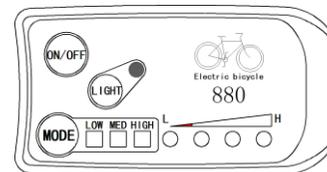
Hold **LIGHT** button shortly to startup the lights (the controller should have the function of headlight driving output or built-in meter headlight driving output function), **LIGHT** indicator lights. Hold **LIGHT** button again to turn off vehicle headlights, and the **LIGHT** indicator is turned off.
