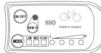
Hold **6KM/H** button and LED indicator flashes, the vehicle drives at the speed should be no more than 6Km/h. Release **6KM/H** button, the function is invalid.
