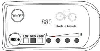
Hold **ON/OFF** button long to startup and enter boot display interface.
